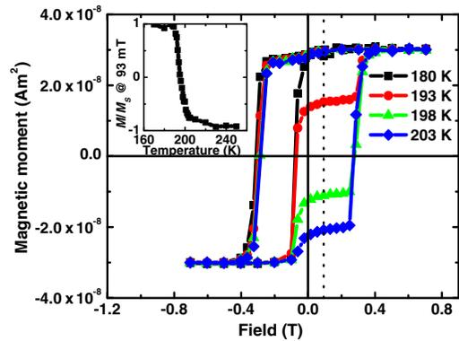
FIG. 1. Hysteresis loops of the magnetization of perpendicular anisotropic Co/Pd for temperatures 180 K (squares), 193 K (circles), 198 K (triangles), and 203 K (diamonds). Diamagnetic background from the substrate is subtracted. Inset: Relative magnetization ( $M/M_s^+$ , magnetization/positive saturation magnetization) at 93 mT (dotted line in the main figure) during the ascending branch of the hysteresis loop.
