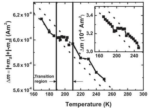
FIG. 3. Total change in the magnetic moment between positive and negative saturation magnetization as a function of the temperature. The transition region is marked. Dotted lines are to guide the eye. Inset shows data of a second piece of the same sample measured with identical protocol.
