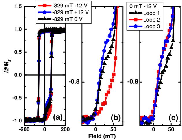
FIG. 4. (a) Hysteresis of sample 2 at 295 K after  $-829$ -mT and  $+12$ -V,  $0$ -V and  $-12$ -V pulses. (b) Detail of the active region shown in (a). (c) Detail of the active region after  $0$  mT and  $-12$  V is pulsed. Loops are taken in succession; each loop is measured in 50 s.
