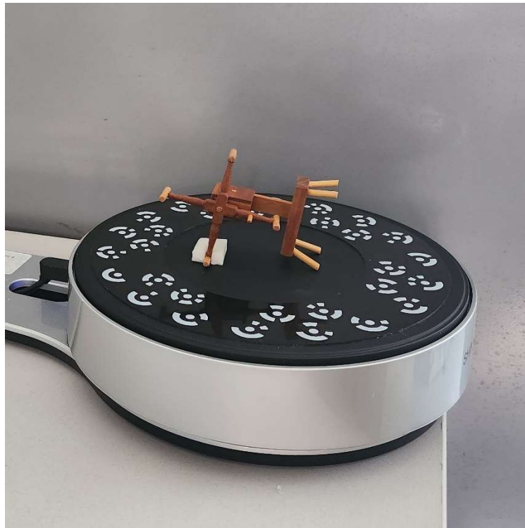
Figure 7: A miniature yarn reel set up on the turntable of the laser scanner used for the project.
