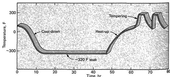
Figure 1: A typical cryogenic treatment cycle [13]
