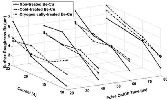
Figure 6: Surface Roughness ( $R_a$ ) results
