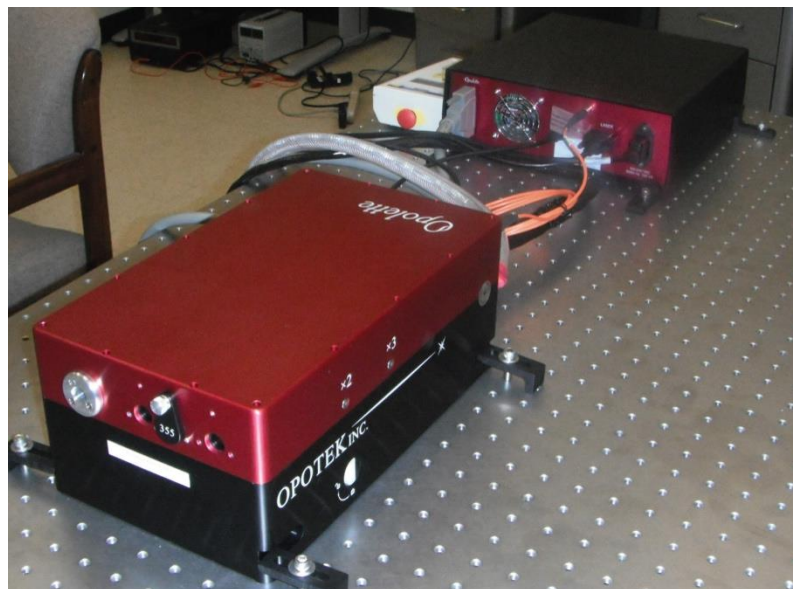
Figure 8: Opolette™ 355 LD pulse laser system incorporated into the SL machine
