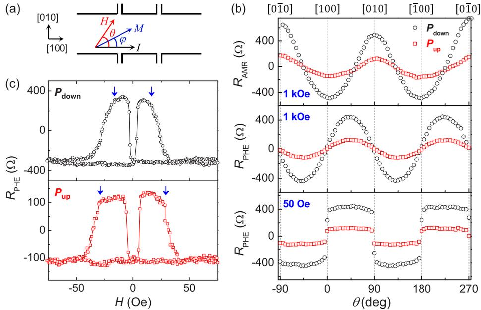
FIG. 2. AMR and PHE taken on a PZT/4 nm LSMO heterostructure. (a) Schematic of the measurement setup. (b)  $\theta$  dependence of  $R_{\text{AMR}}$  at 1 kOe (upper panel),  $R_{\text{PHE}}$  at 1 kOe (middle panel), and 50 Oe (lower panel) at 125 K for both polarization states of PZT. (c)  $R_{\text{PHE}}(H)$  at 125 K for both polarization states. The arrows serve as a guide to the eye.
