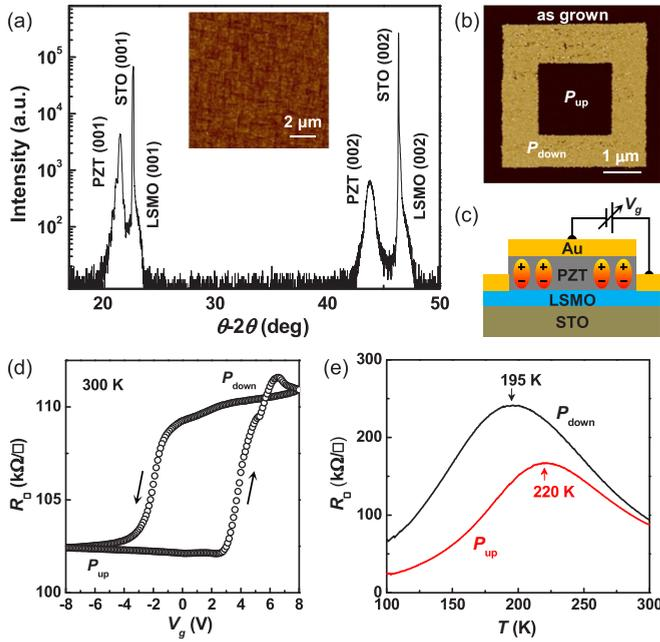
FIG. 1. (a) X-ray  $\theta$ - $2\theta$  scan of a 250 nm PZT/4 nm LSMO on STO. Inset: AFM topography of the sample. (b) PFM phase image of a domain structure written with  $-6$  V ( $P_{\text{up}}$ ) and  $+6$  V ( $P_{\text{down}}$ ) bias voltage applied to a scanning AFM tip. (c) Device schematic. (d)  $R_{\square}(V_g)$  hysteresis taken at 300 K. (e)  $R_{\square}(T)$  for both polarization states, with the corresponding  $T_p$  marked with the arrows.
