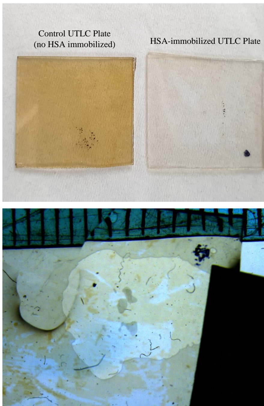
Figure 3.3. ( top image ) Image comparing an undamaged UTLC plate vs. a damaged UTLC plate. ( bottom image ) Magnified picture of damaged UTLC plate. The white streaks are where the nanopillars have been stripped off the glass substrate.
