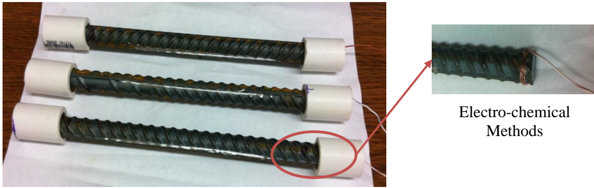
Figure 5.3 Steel rebars' preparation for corrosion tests
