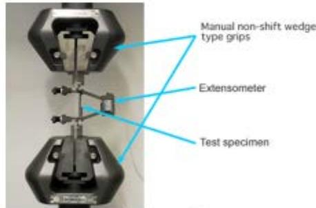
Fig. 2 Test Specimen and Extensometer
