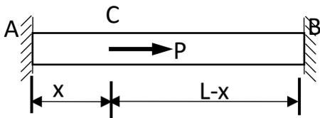
1. (4pts) The axial member has Young's Modulus  $E$ , and cross section area  $A$ . A force  $P$  is acting at the midpoint of the member. Find the displacement at B under the load.
