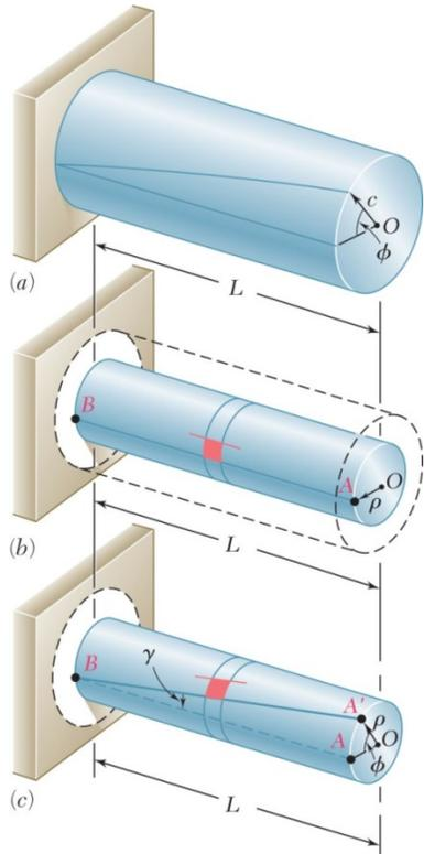
**Shear Stress and Strains Within the Bar**
