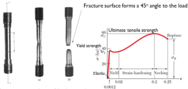
Photo 2.3, 2.4 Tensile test of ductile material specimens: (a) with cross-section necking, (b) ruptured.
