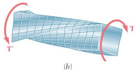
**Shear Strain on surface**
