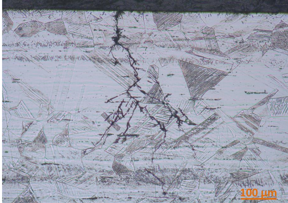
Figure 3.16 Cross-sectional grain morphology of the untreated 304 stainless steel subjected to 72 hours SCC tests. Transgranular and Intergranular cracks were observed.
