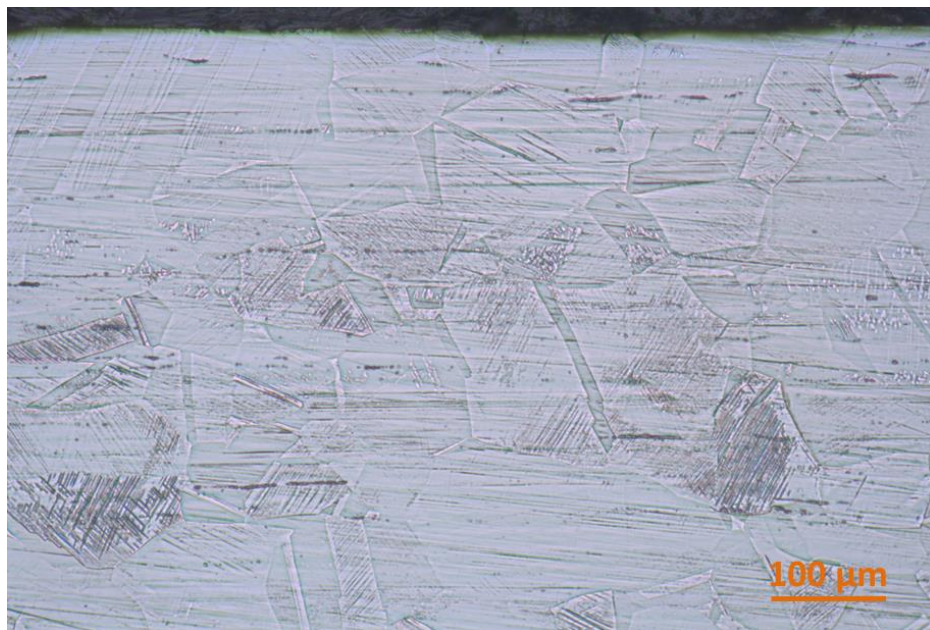
Figure 3.17 Cross-sectional grain morphology of the laser-peened 304 stainless steel subjected to 96 hours SCC tests. No cracks were observed.
