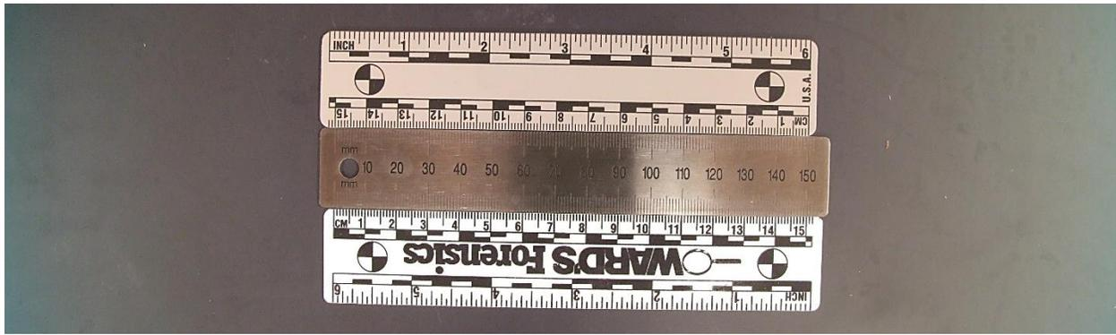
Figure 1: Common commercial scales lined up for comparison to NIST scale.
