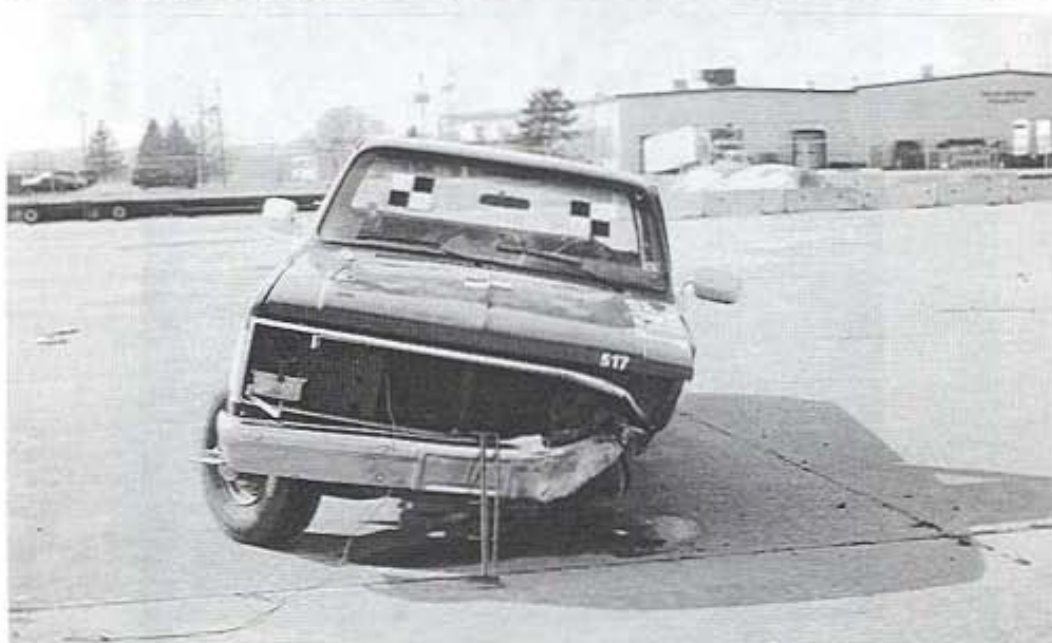
Figure 18. Vehicle Damage, Test ITMP-1
