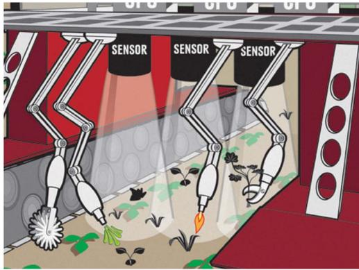
**Figure 2.** Diagram of articulating tools and sensor technologies on a field-based robotic platform for integrated weed control.
