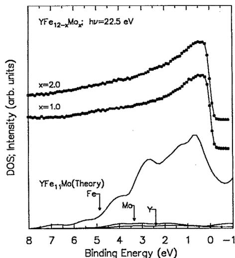
FIG. 1. Calculated partial spin-polarized DOS of Fe, Mo, and Y in  $\text{YFe}_{11}\text{Mo}$  and experimental energy distribution curves (EDC) for clean  $\text{YFe}_{12-x}\text{Mo}_x$  ( $x=1.0, 2.0$ ). The EDCs are normalized to the area under the EDC curves between 0 and 3.5 eV and shifted vertically. The zero on the binding energy axis refers to the Fermi energy ( $E_F$ ).
