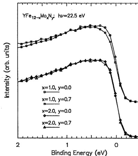
FIG. 2. Expand view of the experimental EDCs of  $\text{YFe}_{11}\text{MoN}_y$  for  $y=0.0, y=0.7$  (upper two curves) and of  $\text{YFe}_{10}\text{Mo}_2\text{N}_y$  for  $y=0.0, y=0.7$  (lower two curves). The zero on the binding energy axis corresponds to the Fermi energy.
