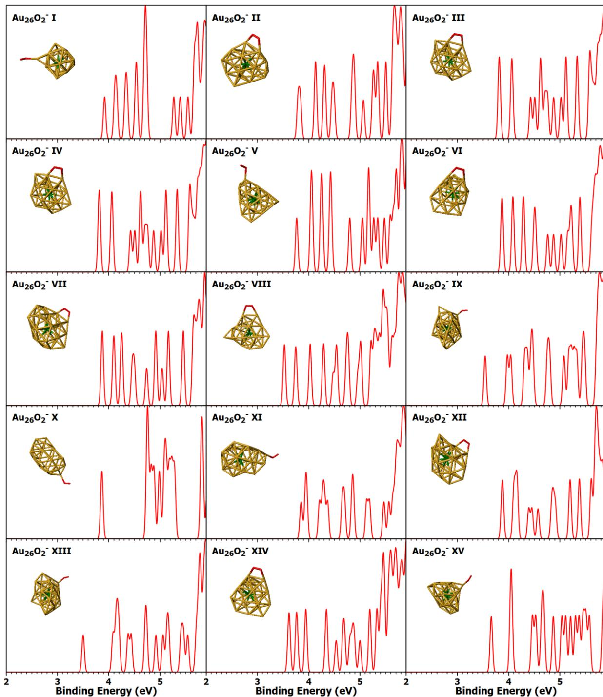
**Figure 7.** Simulated spectra of the low-lying isomers of  $\text{Au}_{26}\text{O}_2^-$ . The gold atoms in green denote the atoms in the core of the cluster. The oxygen molecule is in red.
