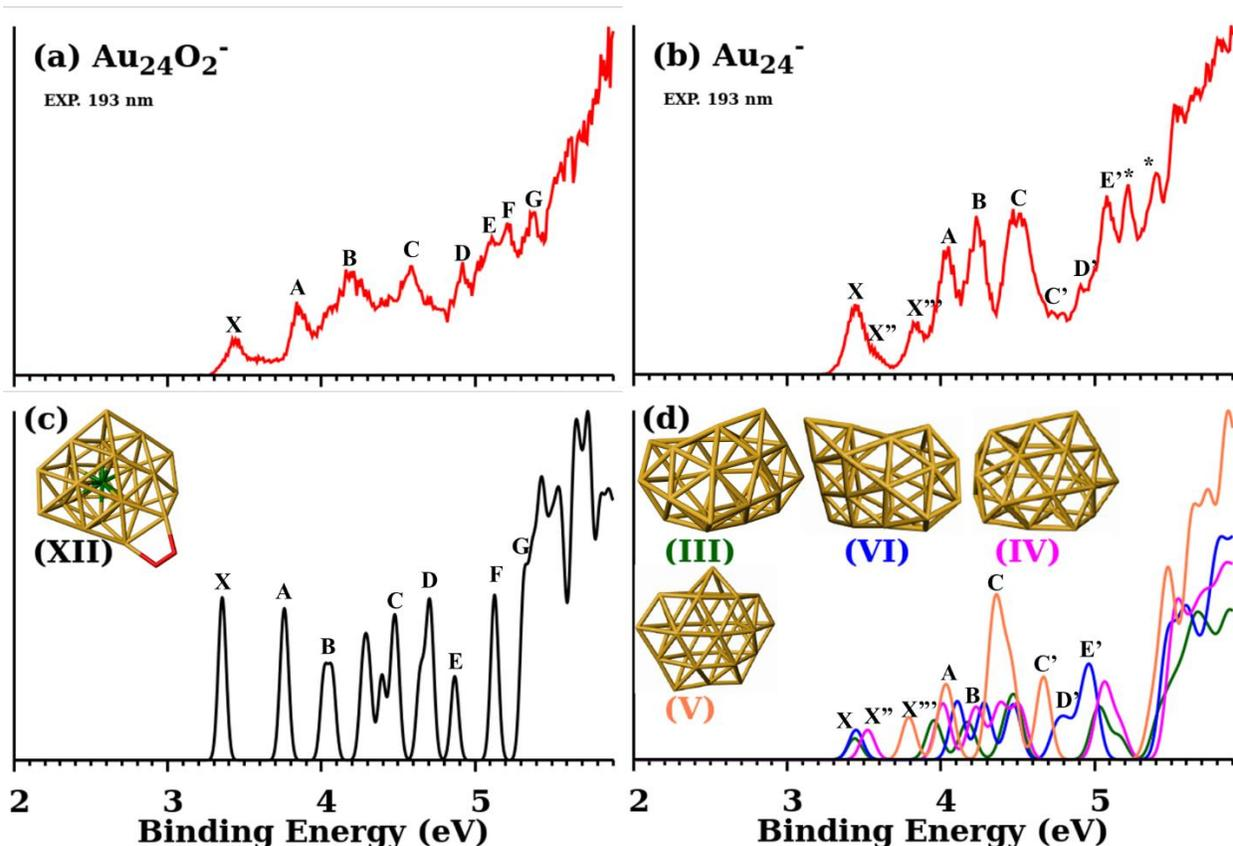
**Figure 3.** Comparison of the simulated spectra (lower panels) with the 193 nm experimental spectra (upper panels) for the low-lying isomers of  $\text{Au}_{24}\text{O}_2^-$  and bare  $\text{Au}_{24}^-$  (see Ref. 57). The gold atom in green denotes the atom in the core of the cluster. The oxygen molecule is in red.
