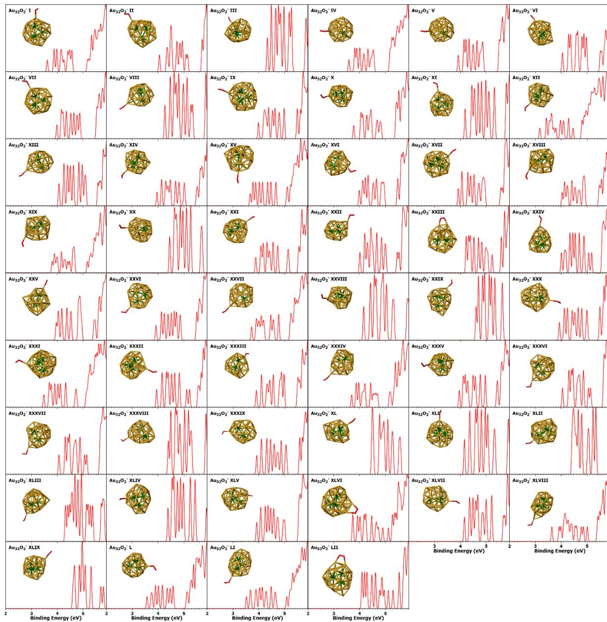
**Figure 10.** Simulated spectra of the low-lying isomers of  $\text{Au}_{32}\text{O}_2^-$ . The gold atoms in green denote the atoms in the core of the cluster. The oxygen molecule is in red.
