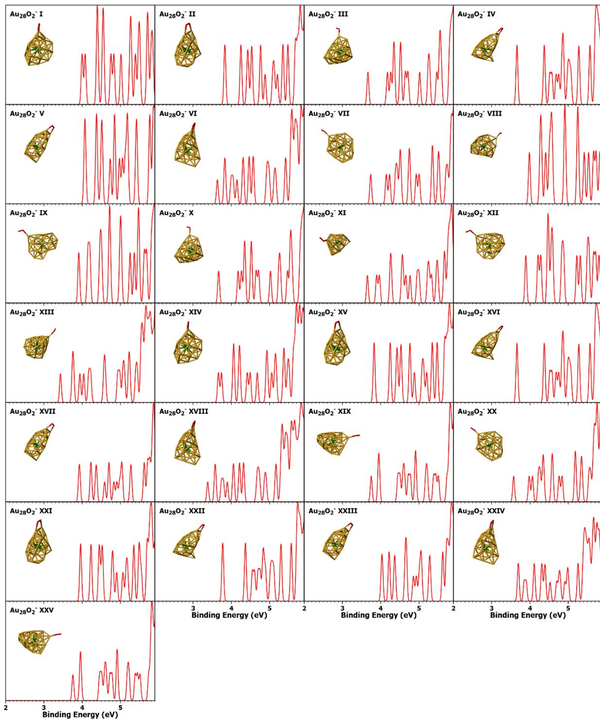
**Figure 8.** Simulated spectra of the low-lying isomers of  $\text{Au}_{28}\text{O}_2^-$ . The gold atoms in green denote the atoms in the core of the cluster. The oxygen molecule is in red.
