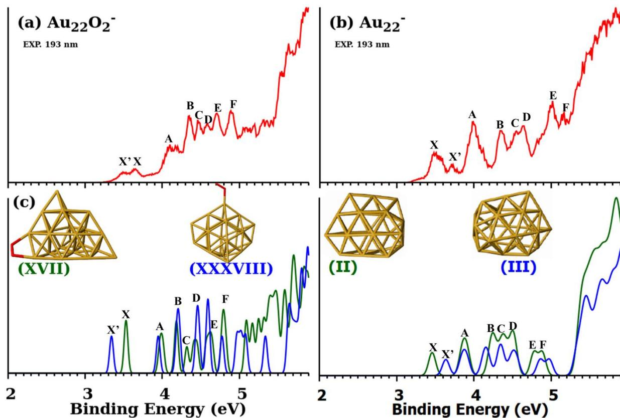
**Figure 2.** Comparison of the simulated spectra (lower panels) with the 193 nm experimental spectra (upper panels) for the low-lying isomers of  $\text{Au}_{22}\text{O}_2^-$  and bare  $\text{Au}_{22}^-$  (see Ref. 57). The oxygen molecule is in red.
