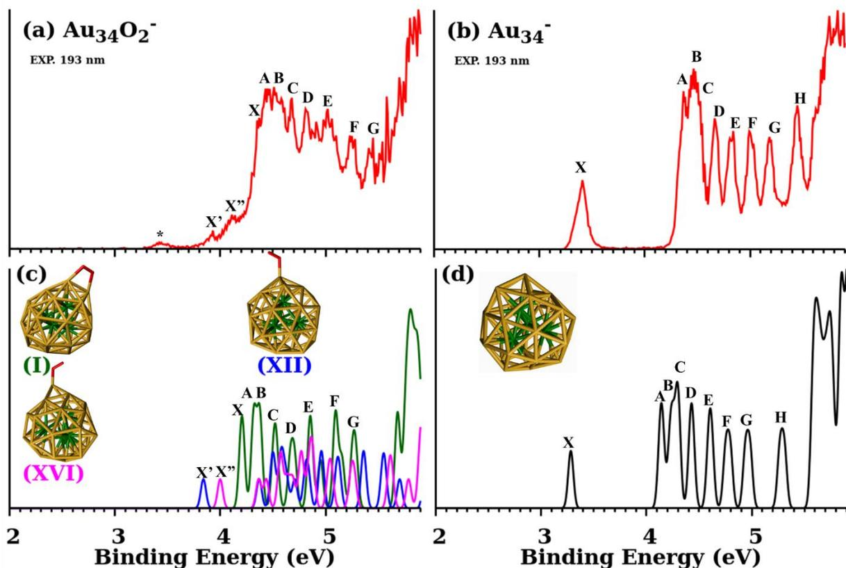
**Figure 4.** Comparison of the simulated spectra (lower panels) with the 193 nm experimental spectra (upper panels) for the low-lying isomers of  $\text{Au}_{34}\text{O}_2^-$  and bare  $\text{Au}_{34}^-$  (see Ref. 81). The gold atoms in green denote the atoms in the core of the cluster. The oxygen molecule is in red.
