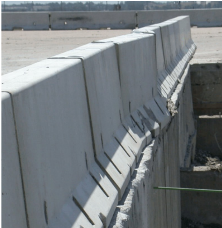
Figure 25. System Damage, Test KTB-1
