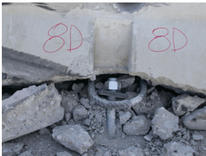
Figure 28. Barrier No. 8 Tie-Down Anchor Damage, Test KTB-1
