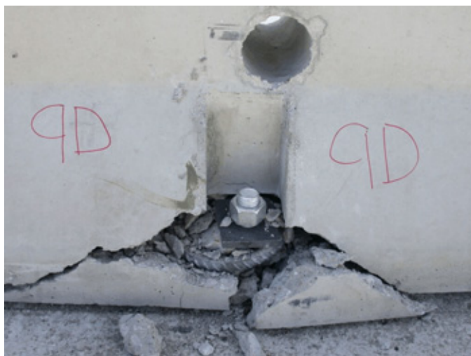
Figure 29. Barrier No. 9 Tie-Down Anchor Damage, Test KTB-1
