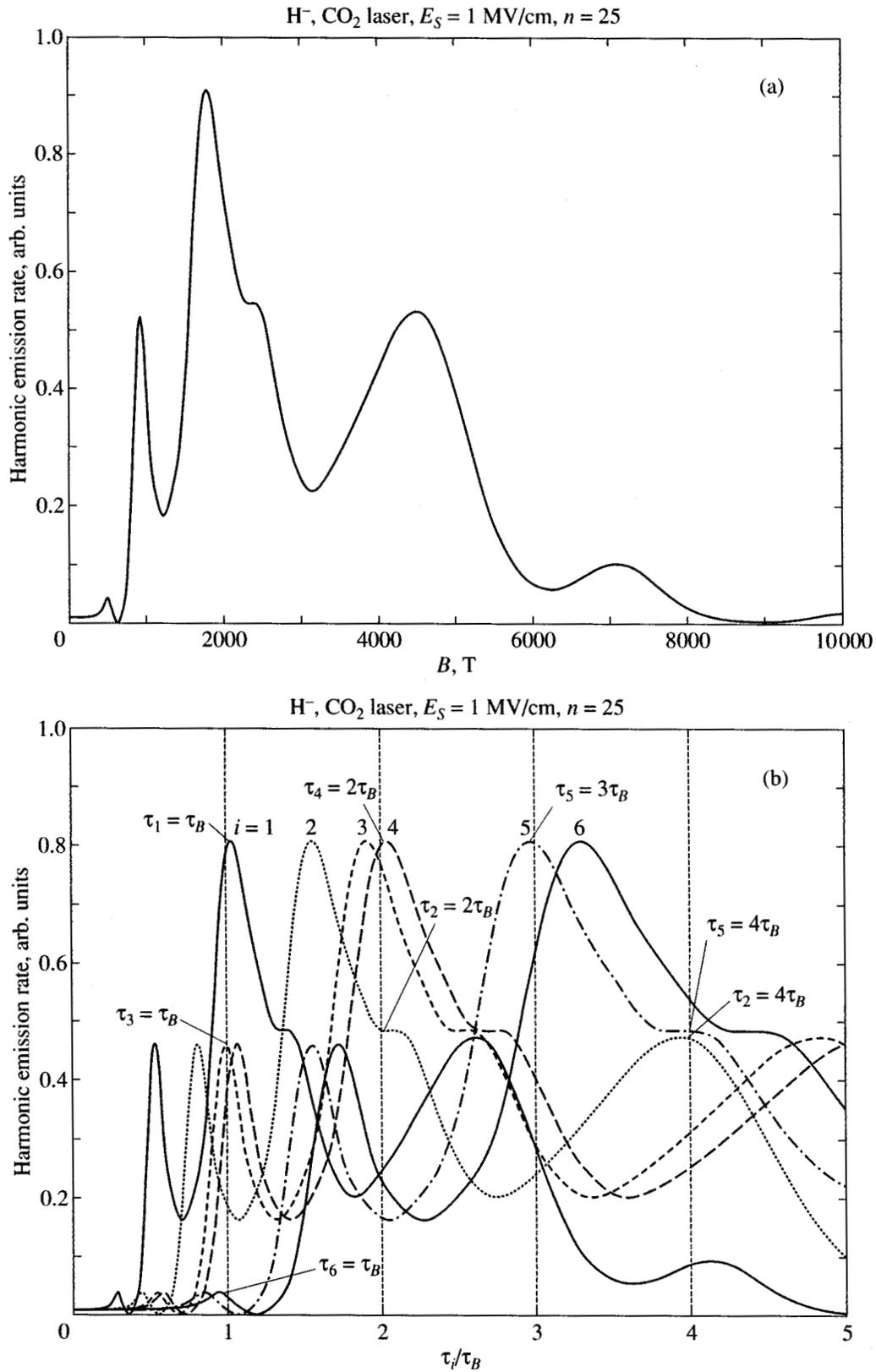
**Fig. 12.** The 25th harmonic emission rate as a function of the magnetic field induction  $B$  for the same parameters as in Fig. 11. (a) Emission rate plotted vs.  $B(\tau)$ . (b) Emission rate plotted vs. the dimensionless parameters  $\tau_i/\tau_B$ ,  $i = 1, \dots, 6$ , where  $\tau_i$  is the  $i$ th classical return time. The harmonic emission rate has maxima for  $\tau_i = j\tau_B$ , where  $i$  and  $j$  are integers, and  $\tau_B$  is the cyclotron period.
