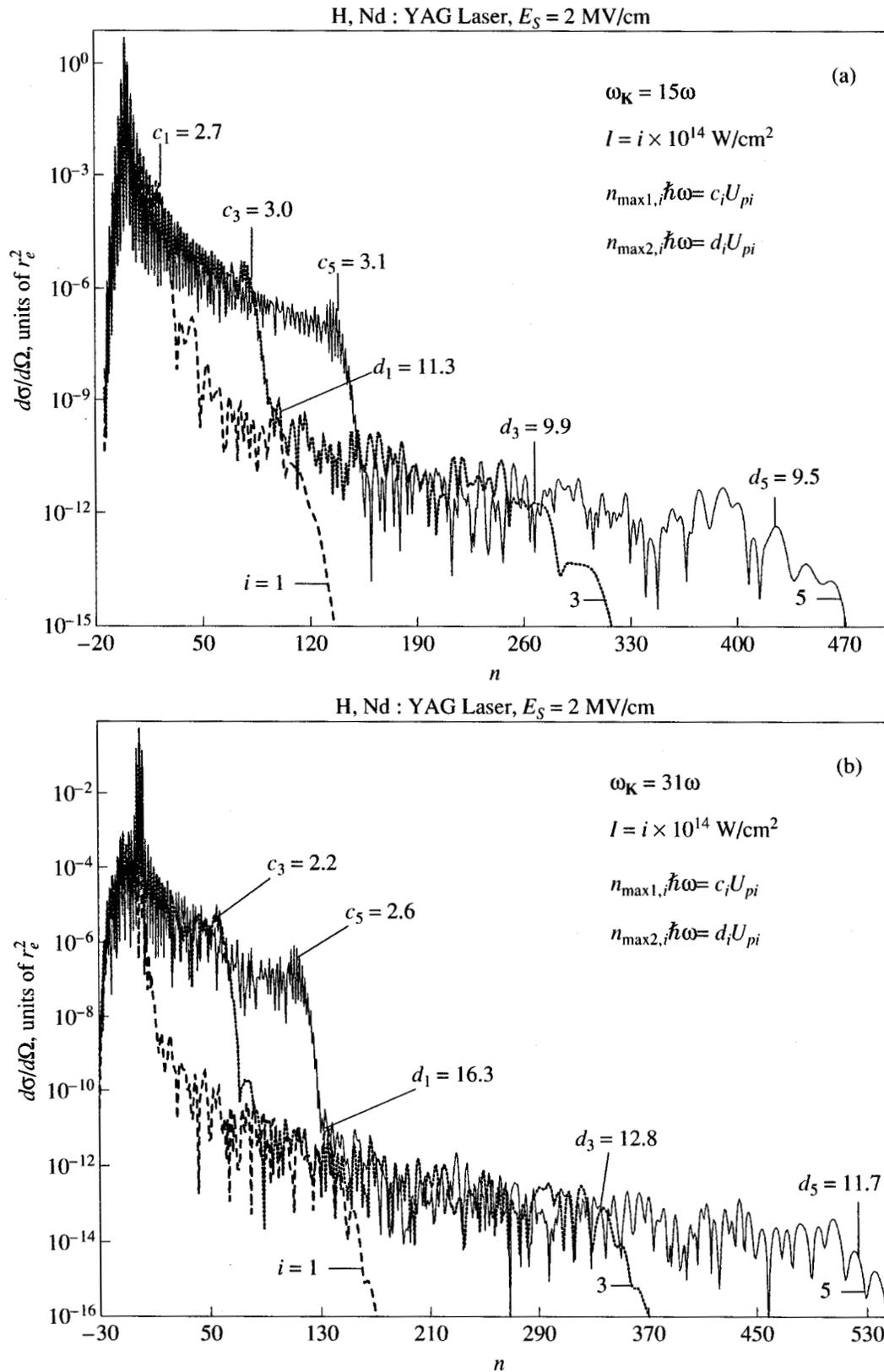
**Fig. 7.** The same as in Fig. 6, but in the presence of an additional static electric field having strength  $E_S = 2$  MV/cm, and for laser intensities  $I(i) = i \times 10^{14} \text{ W/cm}^2$ , where  $i = 1, 3,$  and  $5$ . The energy cutoff positions for higher and lower DCS plateaus are denoted by the ponderomotive energy multiples  $c_i$  and  $d_i$ , respectively.
