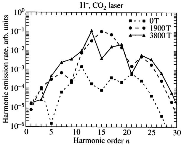
**Fig. 8.** Harmonic emission rates as functions of the harmonic order  $n$  for the  $H^-$  ion and a  $CO_2$  laser with intensity  $I = 5 \times 10^{10} \text{ W/cm}^2$ . The magnetic field induction is:  $B = 0 \text{ T}$  (squares),  $1900 \text{ T}$  (circles), and  $3800 \text{ T}$  (triangles).
