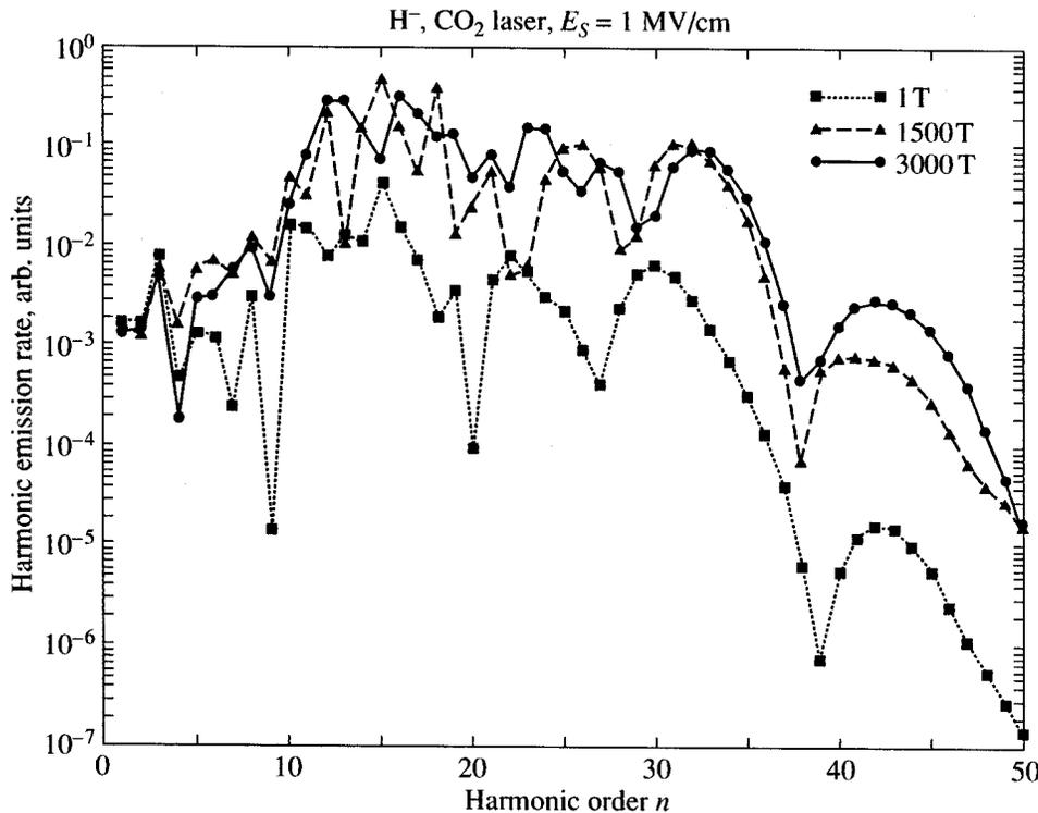
**Fig. 9.** The same as in Fig. 8, but in the presence of a parallel static electric field having strength  $E_S = 1 \text{ MV/cm}$ , and for the following values of the magnetic field induction:  $B = 1 \text{ T}$  (squares),  $1500 \text{ T}$  (triangles), and  $3000 \text{ T}$  (circles).
