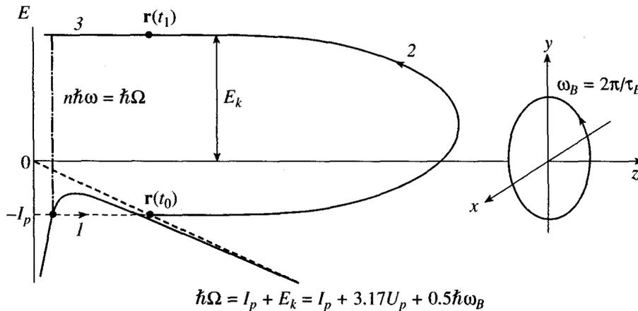
**Fig. 1.** Schematic of high-harmonic generation in the presence of a magnetic field. The laser field is linearly polarized along the  $z$ -axis. Numbers 1, 2, and 3 denote the steps of the three-step model. The  $E$ -axis denotes the electron energy coordinate, and  $\omega_B$  is the cyclotron frequency for the electron's (perpendicular) motion in the  $xy$ -plane. See the text for a more detailed explanation.
