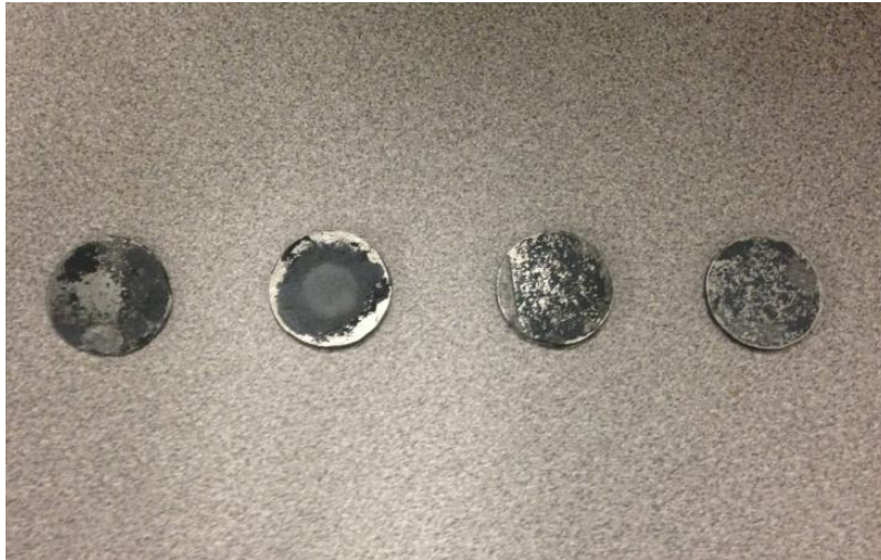
Figure 2.3: The sample surfaces covered with graphite layers
