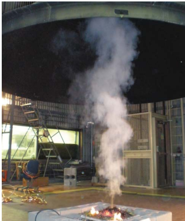
Laboratory burns assisted in creating smoke profiles of various fuel types.
