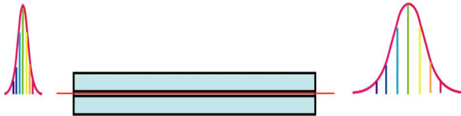
Fig. 2. 17: Pulse spreading due to chromatic dispersion (CD) [95].
