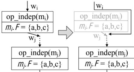
Figure 4: Merge Identical Subsequent Operator
