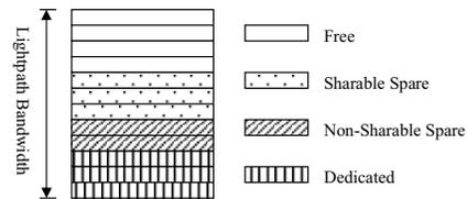
Fig. 5. Classification of channels within a lightpath.
