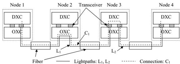
Fig. 1. Illustration of lightpaths and a connection in traffic grooming. Lightpath  $L_1$  traverses fiber link (1,2) and (2,3), lightpath  $L_2$  traverses fiber link (3,4), and connection  $C_1$  uses a two-hop path using lightpaths  $L_1$  and  $L_2$ .
