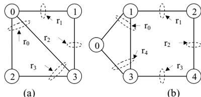
Fig. 8. (a) Network 1: a 4-node network. (b) Network 2: a 5-node network. The links covered by a dashed circle belong to the same SRLG.
