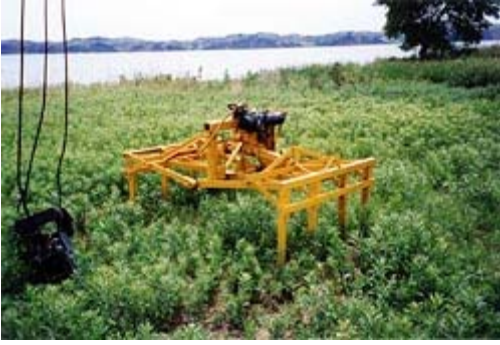
Figure 4. Commercially manufactured hay bale tongs for a crane. Were these actually attached to a crane, they would be hydraulically operated from inside the cab. Lake Sharpe, South Dakota, June, 1994.
