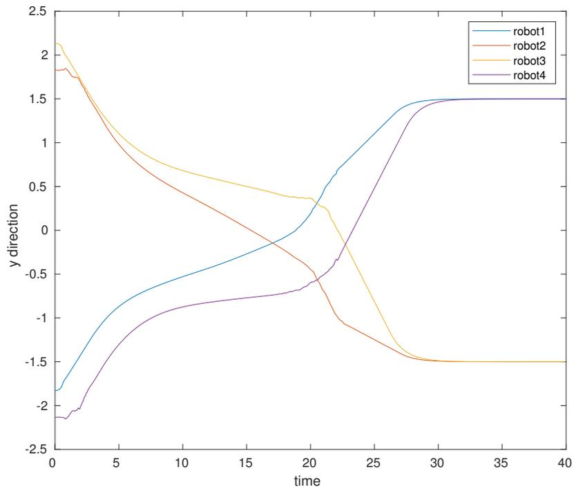
Figure 6.4: The y direction trajectory of each robot
