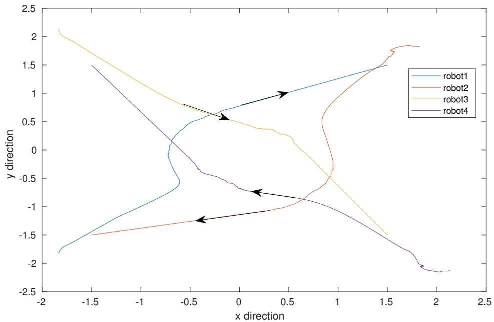
Figure 6.7: The trajectory of each robot with kinematics constraints
