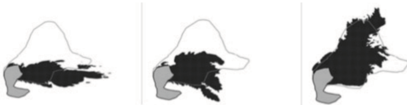
This graphic shows fire growth predictions from the model reconstructions of the 1994 South Canyon Fire, west of Glenwood Springs, Colorado. The uniform wind field is on the left, the WindNinja wind field in the center, and the WindWizard wind field at right.
