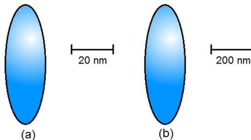
FIG. 1. Shape anisotropy and size scaling. Both magnets are made from the same materials and have the same shape, but the coercivity of (b) is about 100 times smaller than that of (a).
