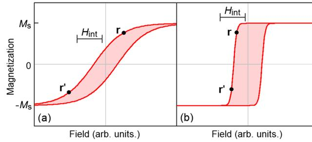
FIG. 3. Cooperative phenomena on the hysteresis loop: (a) noncooperative and (b) cooperative. Cooperativity means the interaction field  $H_{\text{int}}$  between two magnetic regions at  $\mathbf{r}$  and  $\mathbf{r}'$  is larger than the difference in the switching fields of the regions.
