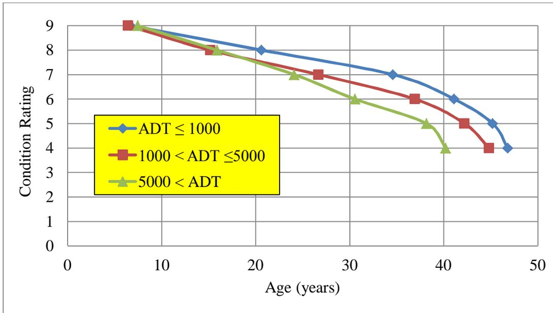
Figure 4-1: Original deck deterioration curve in state bridges
