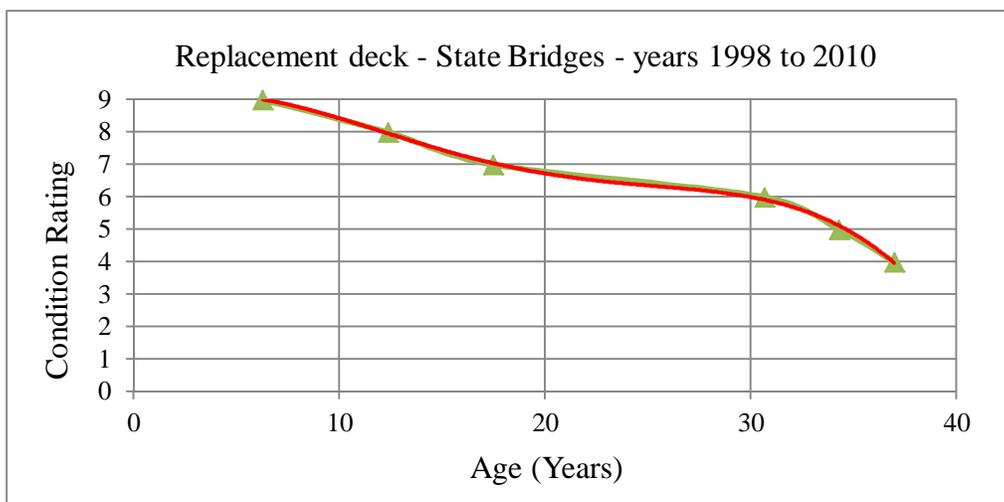
Figure 4-6: Replacement deck deterioration curve in state bridges
