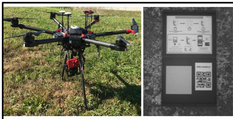
Figure 2. 4. DJI Matrice 600 attached MicaSense Rededge multispectral and FLIR Duo Pro R thermal sensors (Left) and MicaSense calibration redlectance panel (Right).
