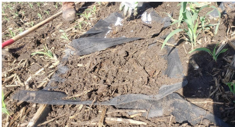
Figure 2.3. Fabric and mesh bag burial in research plots
