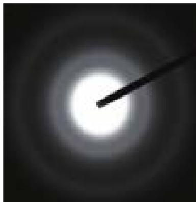
*Fig. 2.9: Selected Area Electron Diffraction (SAED) pattern obtained from silica superstructures showing amorphous halos. Reprinted with permission from [13].*
