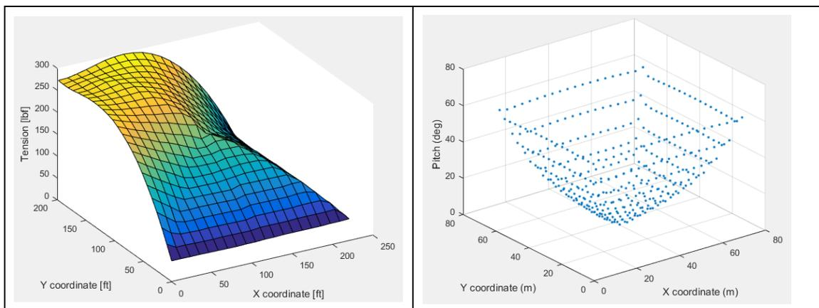
Figure 2-3. Model mesh outputs. (left) Theoretical cable tension. (right) Theoretical end-effector pitch.
