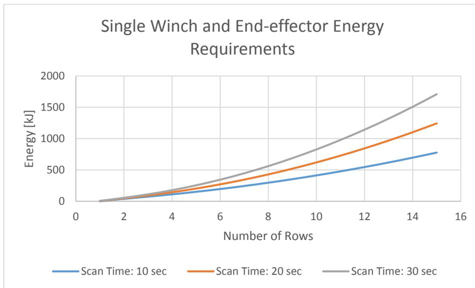
Figure 6-12. Single winch and end-effector energy requirements.
