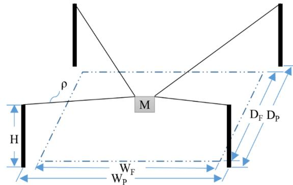
Figure 2-4. System parameters of a four-cable CDRP system.
