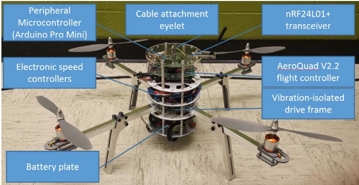
Figure 5-1. AeroQuad-based IPASS prototype. Tethers not shown.
