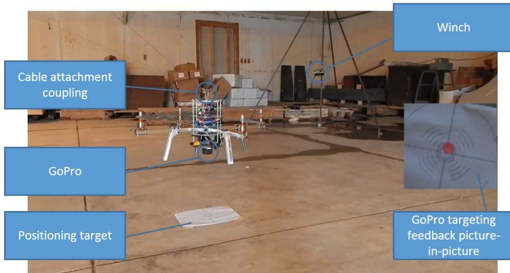
Figure 5-2. IPASS prototype experimentation video snapshot.<sup>9</sup>
