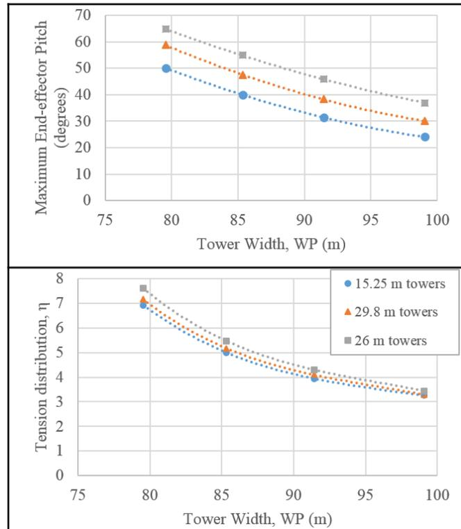
Figure 2-6. Dimensional considerations. (top) Theoretical end-effector pitch. (bottom) Theoretical tension distribution.
