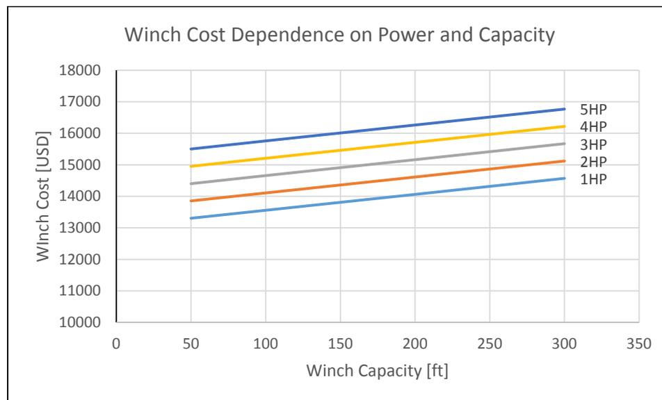
Figure 6-4. Winch cost dependence on power and capacity.
