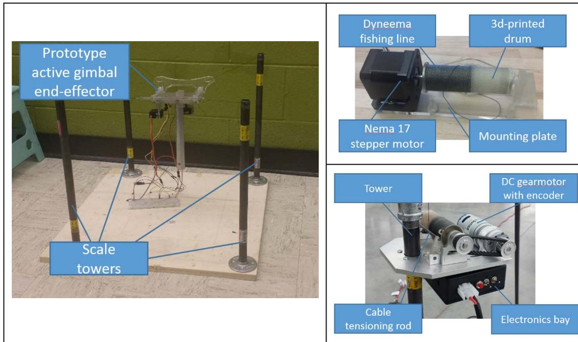
Figure 3-1. CDPR model components. (left) Desktop prototype. (right-top) Initial winch design using stepper motor. (right-bottom) Current CPDR winch, using DC gearmotor and encoder.
