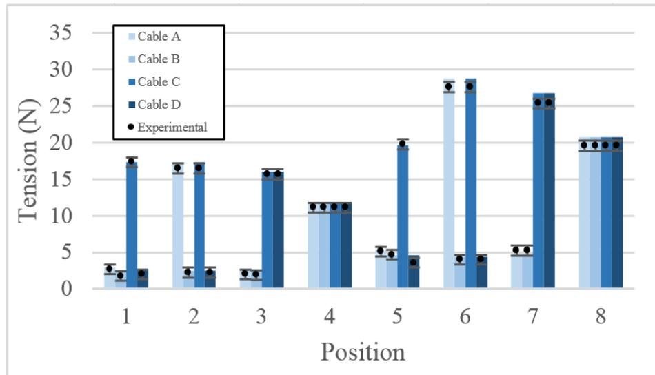
Figure 4-3. Theoretical vs. experimental cable tensions.<sup>7</sup>
