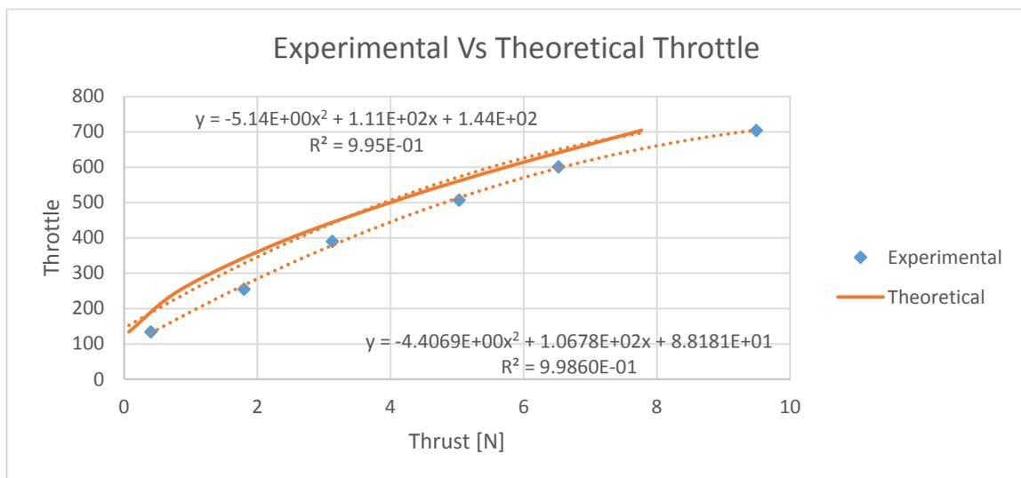
Figure 5-8. Experimental vs. theoretical throttle-thrust curves.
