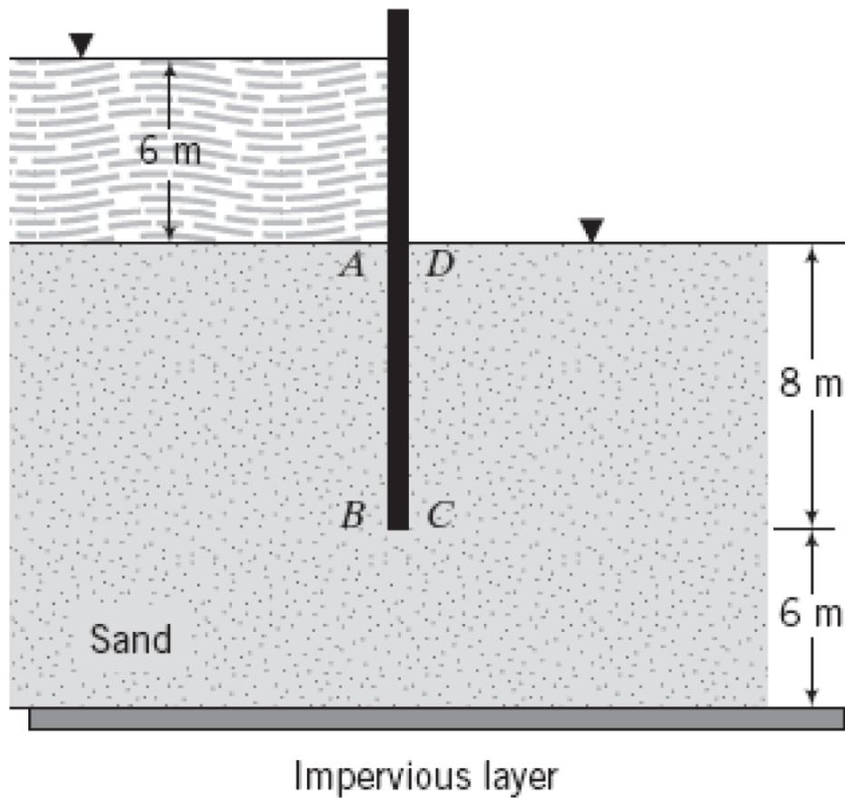
What is the ratio of the number of flow channels ( $N_f$ ) to the number of potential drops ( $N_d$ )?
