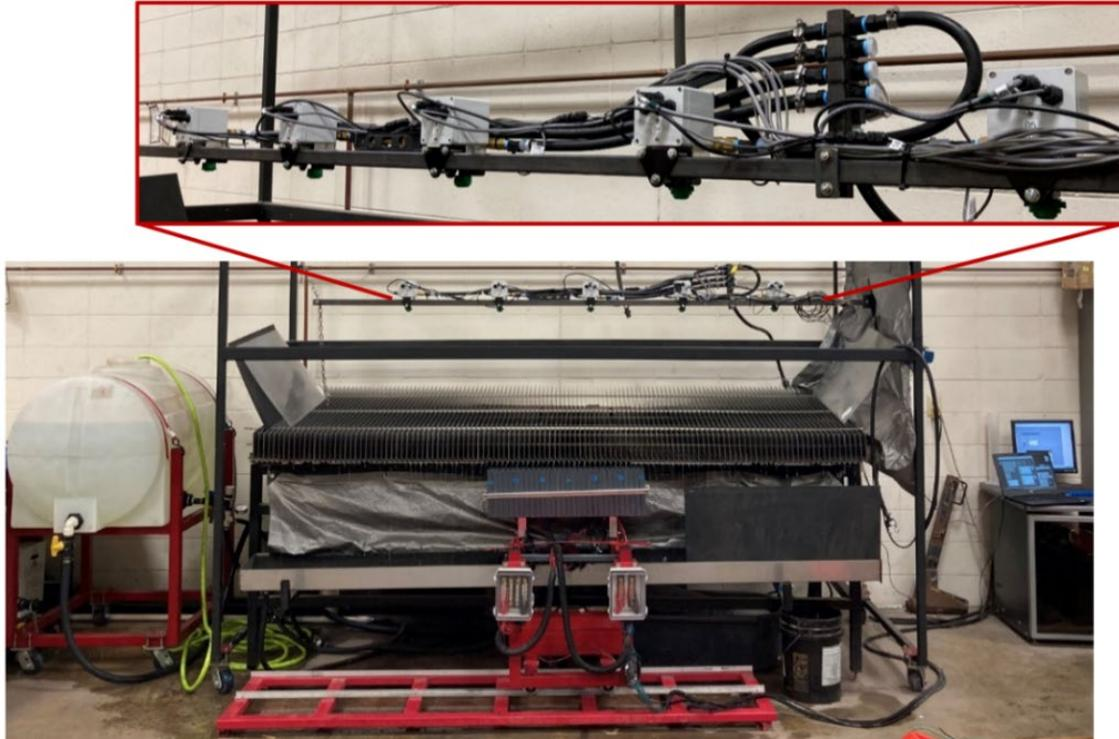
Figure 21 - Nozzles installed on patternator at W. F. Splinter Labs.
