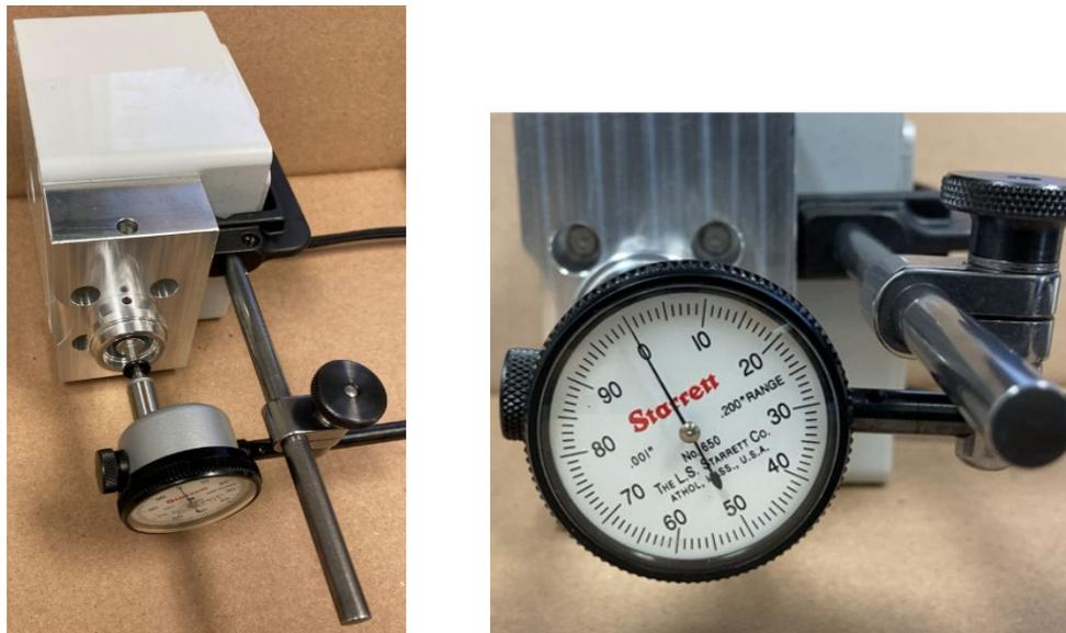
Figure 16 - Dial indicator set up to measure nozzle metering stem displacement.
