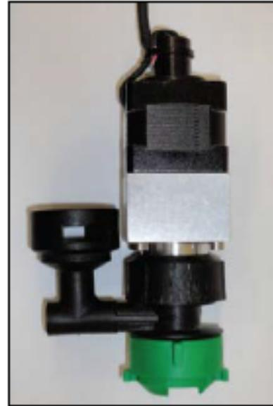
Figure 3 – Prototype electromechanical variable-orifice spray nozzle.
