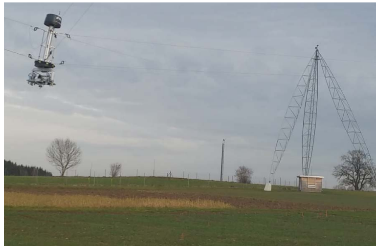
Figure 1-10. ETH end-effector experiencing tilt as it approaches the edge of workspace.
