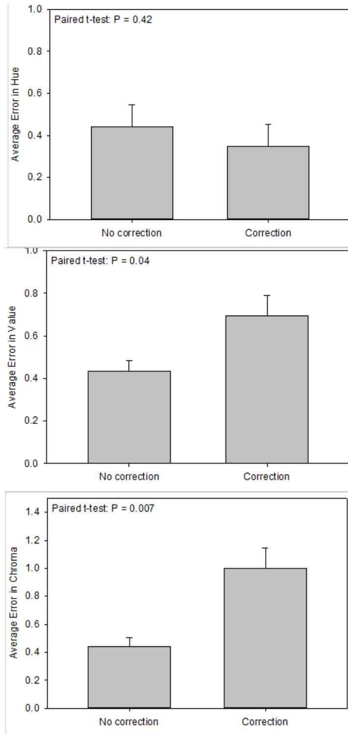
Fig. 3. Results of soil color lab, showing changes in student errors in hue, value, and chroma in response to corrections made using the visual color adjustment guide prepared by comparing their soil color readings to the chroma meter-determined colors.
