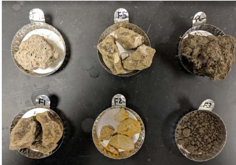
Fig. 7. Hand specimens used in the lab practical displaying: F1) manganese films, F2) redoximorphic concentrations and depletions, F3) granular structure, F4) vesicular pores, F5) carbonate nodules, F6) subangular blocky structure.
