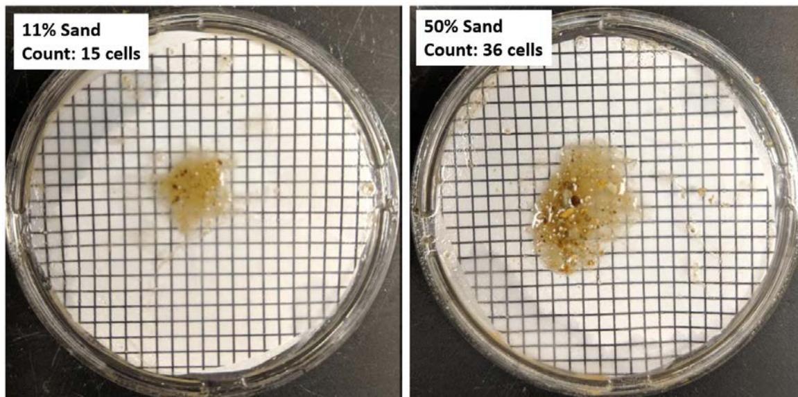
Fig. 10. Grid disc containing sands washed from samples with 11% and 50% sand.
