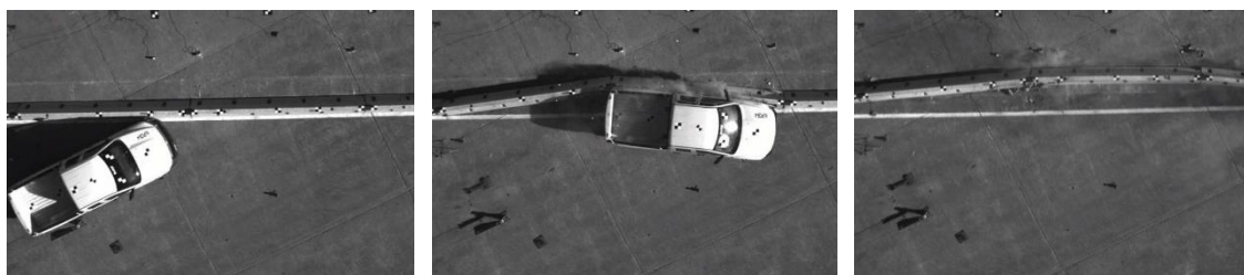
Figure 30. Barrier Deflection (Impact location, during impact, and Post Impact)
