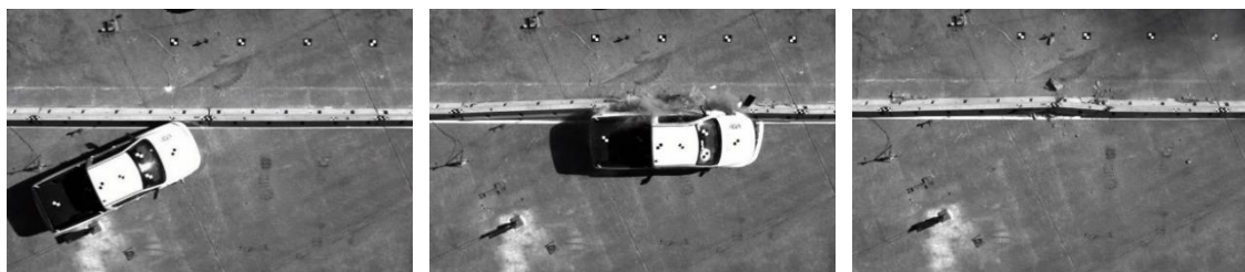
Figure 18. Barrier Deflection (Impact location, during impact, and Post Impact)
