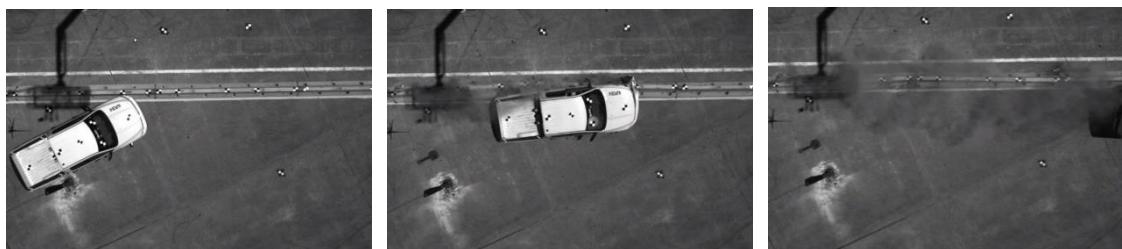
Figure 38. Barrier Deflection (Impact location, during impact, and Post Impact)
