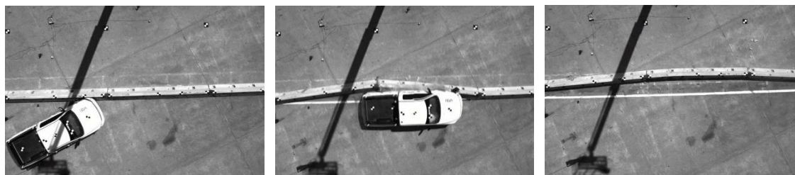
Figure 26. Barrier Deflection (Impact location, during impact, and Post Impact)
