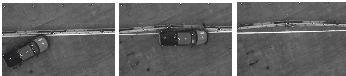
Figure 34. Barrier Deflection (Impact location, during impact, and Post Impact)
