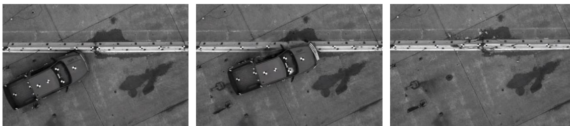
Figure 22. Barrier Deflection (Impact location, during impact, and Post Impact)
