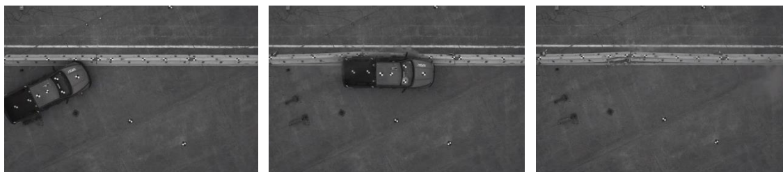
Figure 42. Barrier Deflection (Impact location, during impact, and Post Impact)
