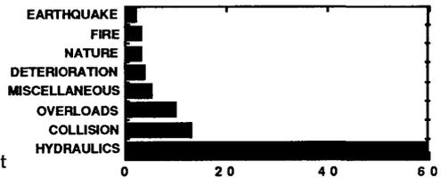
Figure 1.-- Percent of bridge failures by failure mode
