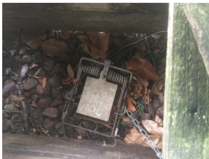
Top: Ideal location for a trap box. Rats can't resist exploring holes Bottom: Trap set in box - the middle panel of the box lifts off to allow you to check the trap without putting your scent on the main box.
