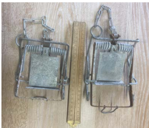
Top left: Fenn type traps come in two sizes. The smaller Mark IV is fine for rats and weasels, but would struggle to kill an adult Mink. If there are mink in your area, the Mark VI would be safer. Bottom left: Fenn Mark IV set - notice that the safety catch beside the brass bar has been moved back to allow the trap to close. Photos: Ian Clark
