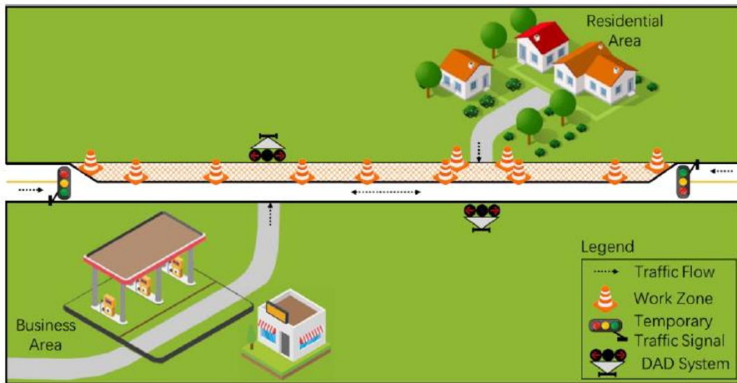
Figure 1.1 A Typical layout of a DAD system with temporary traffic control signals
