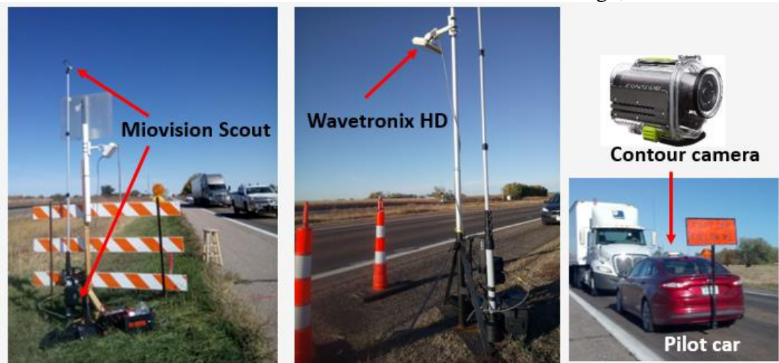
(c) Data collection devices installed at the work zone test sites
