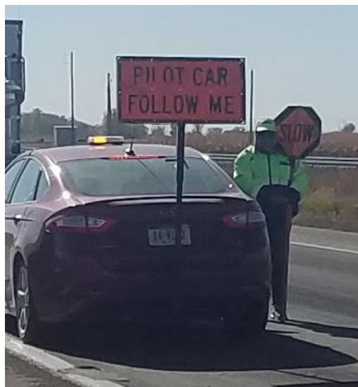
Figure 2.3 A typical pilot car for work zone traffic control
