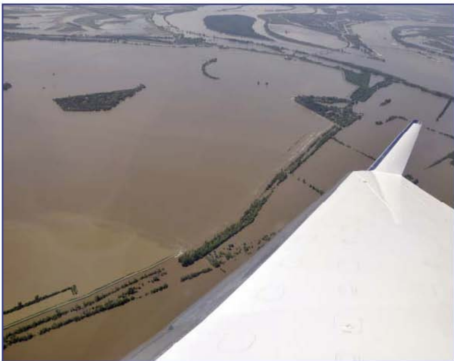
Below: Aerial view of the upper crevasse site after activation of the floodway.
