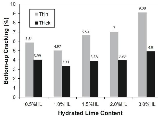
Figure 10. MEPDG predictions of pavement bottom-up cracking.
