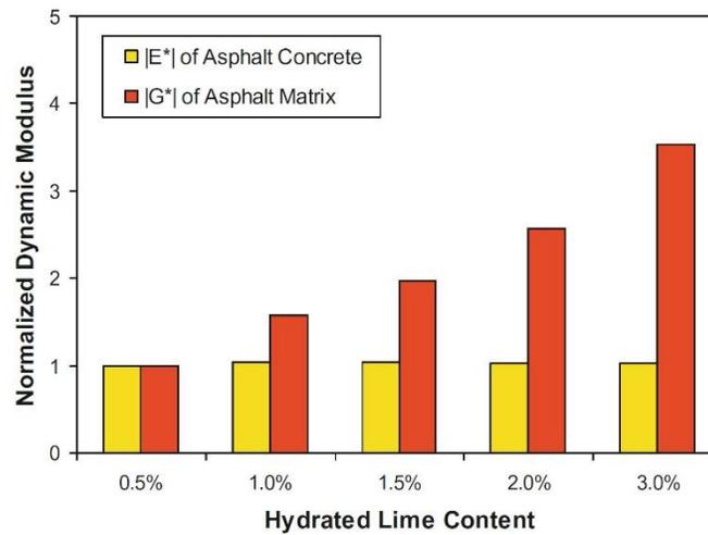
Figure 5. Normalized dynamic moduli of mixtures at 10 Hz.
