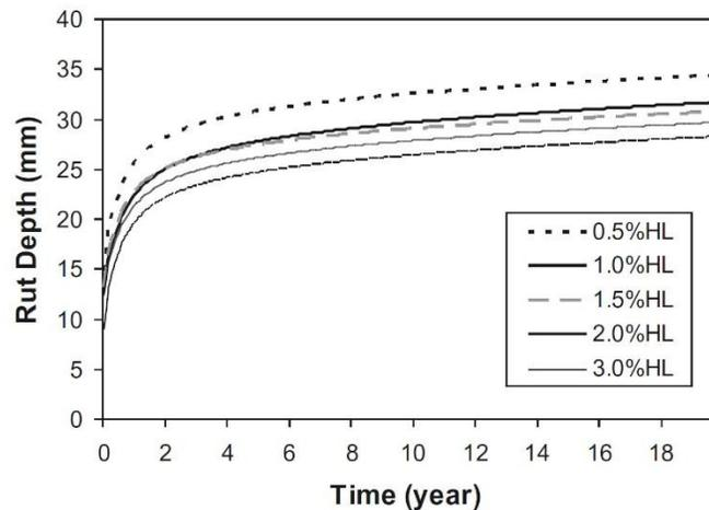
**Figure 9.** MEPDG predictions of pavement rut depth.
