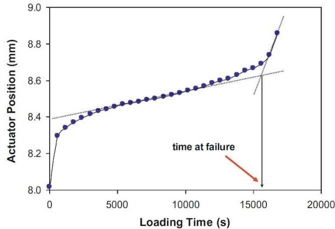
Figure 3. An example plot of the IDT permanent deformation test at 60°C.
