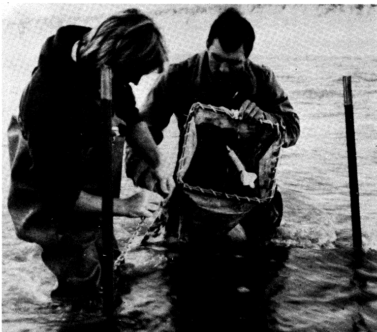
Research biologists prepare a specially-designed drift net for a typical set. The flowmeter in the mouth of the net quantified the ichthyoplankton samples.
