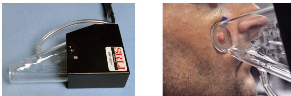
Figure 1. Left: Glass chamber used to create vacuum and measure displacement with skin or elastomer. Right: Vacuum applied to facial skin, with displacement measured by movement of laser target, which is seen as a red dot in the center of displaced skin.
