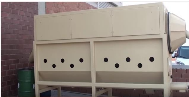
Video 3 1 ton pomace separator, marc separator. Separates grape seed from grape skin, Onmak Makina.
