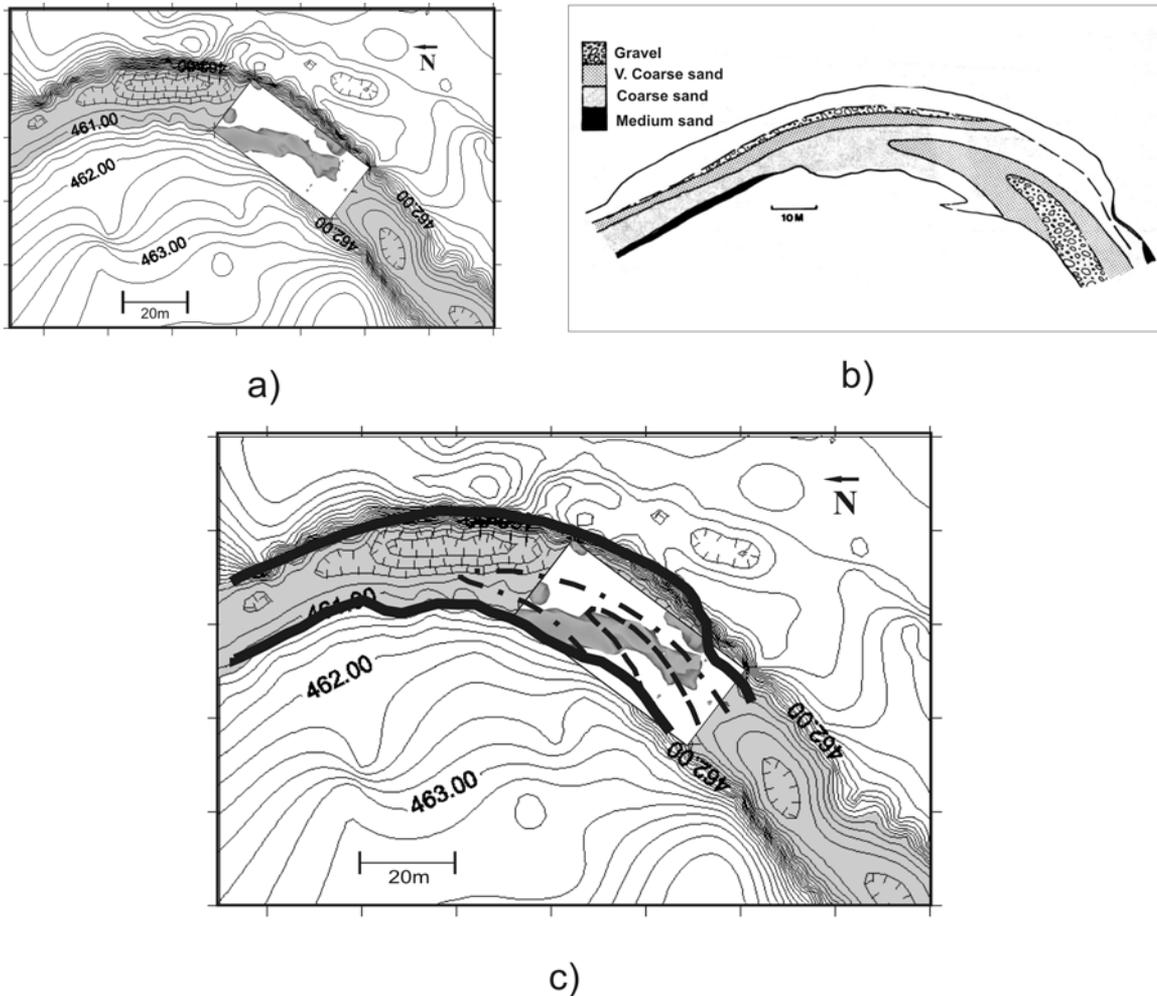
**Figure 8.** Comparison of channel bend deposits: (a) Prairie Creek data based on CHIT; (b) channel bend deposits as observed on River South Esk, Scotland (modified from *Bridge* [1977], reprinted with permission of John Wiley); (c) is a superposition of Figures 8a and 8b. Solid lines represent the river banks, dashed-dotted lines bound very coarse sand deposits, and dashed lines bound gravel deposits.
