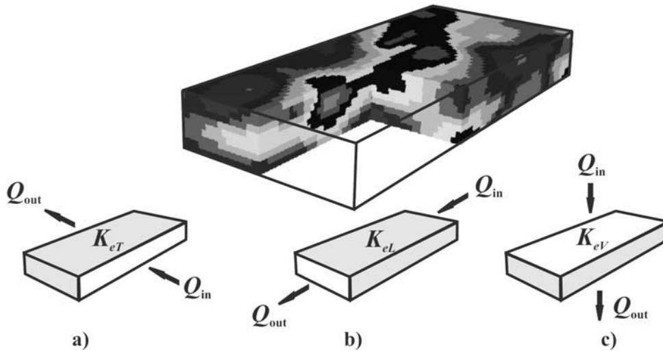
**Figure 6.** MODFLOW models used for calculating effective  $K$  in different directions. Gray-shaded boundaries are no-flow boundaries, clear faces are constant-head boundaries. (a)  $K_{eT} = 18.5$  m/d - transverse case, (b)  $K_{eL} = 19.5$  m/d - longitudinal case, and (c)  $K_{eV} = 18.1$  m/d - vertical case. See color version of this figure at back of this issue.
