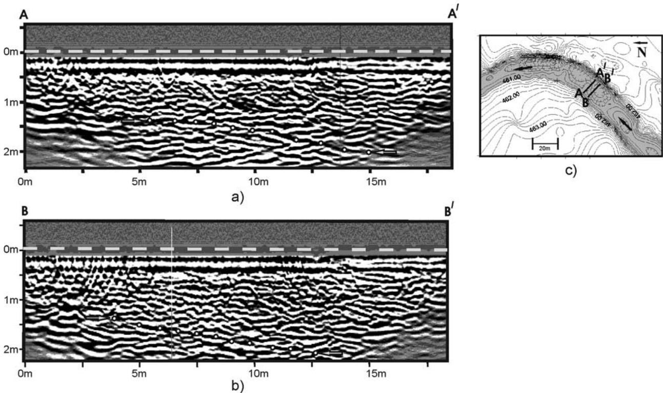
**Figure 12.** GPR profiles across the Prairie Creek 1.5 m apart: (a) downstream section A-A'; (b) upstream section B-B'; (c) location of GPR profiles. Arrows in Figures 12a and 12b point to ends of semicontinuous reflector (traced by a series of open circles) interpreted as a major scour surface dipping toward the direction of the cutbank.
