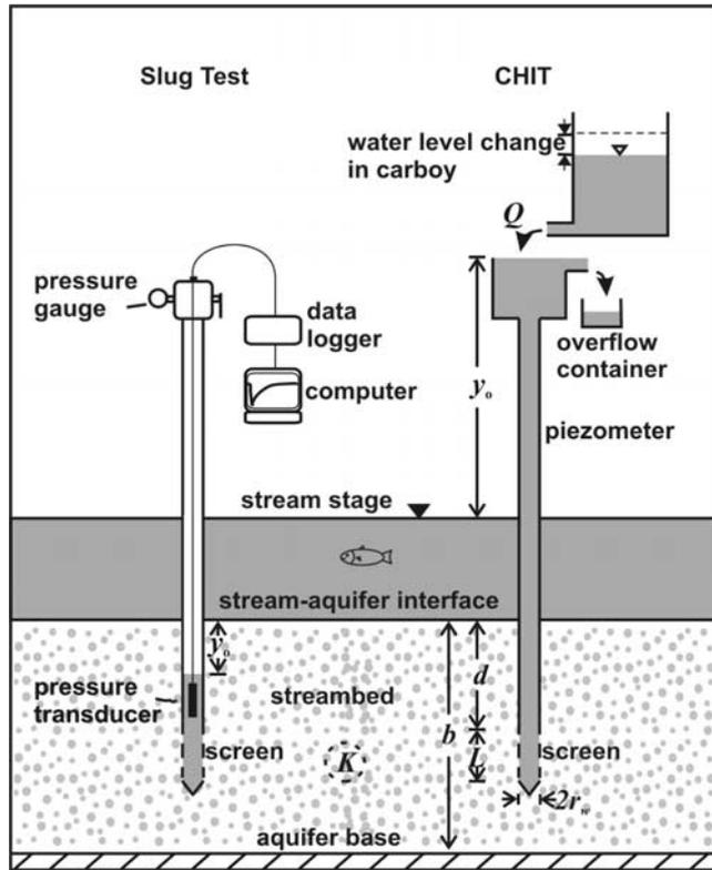
Figure 2. Schematic representation of slug test and CHIT.
