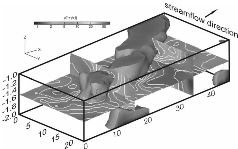
**Figure 7.** Three-dimensional hydraulic conductivity field generated through kriging of  $K$ . Shaded arcuate region corresponds to  $K$  of  $\geq 30$  m/d. Note vertical exaggeration:  $10\times$  and that inset color legend is logarithmic.  $K$  isoline interval on sections is 5 m/d. Axes are in meters. See color version of this figure at back of this issue.
