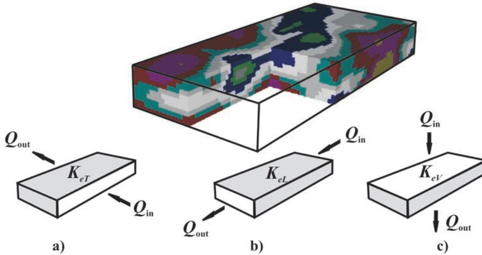
**Figure 6.** MODFLOW models used for calculating effective  $K$  in different directions. Gray-shaded boundaries are no-flow boundaries, clear faces are constant-head boundaries. (a)  $K_{eT} = 18.5$  m/d - transverse case, (b)  $K_{eL} = 19.5$  m/d - longitudinal case, and (c)  $K_{eV} = 18.1$  m/d - vertical case.
