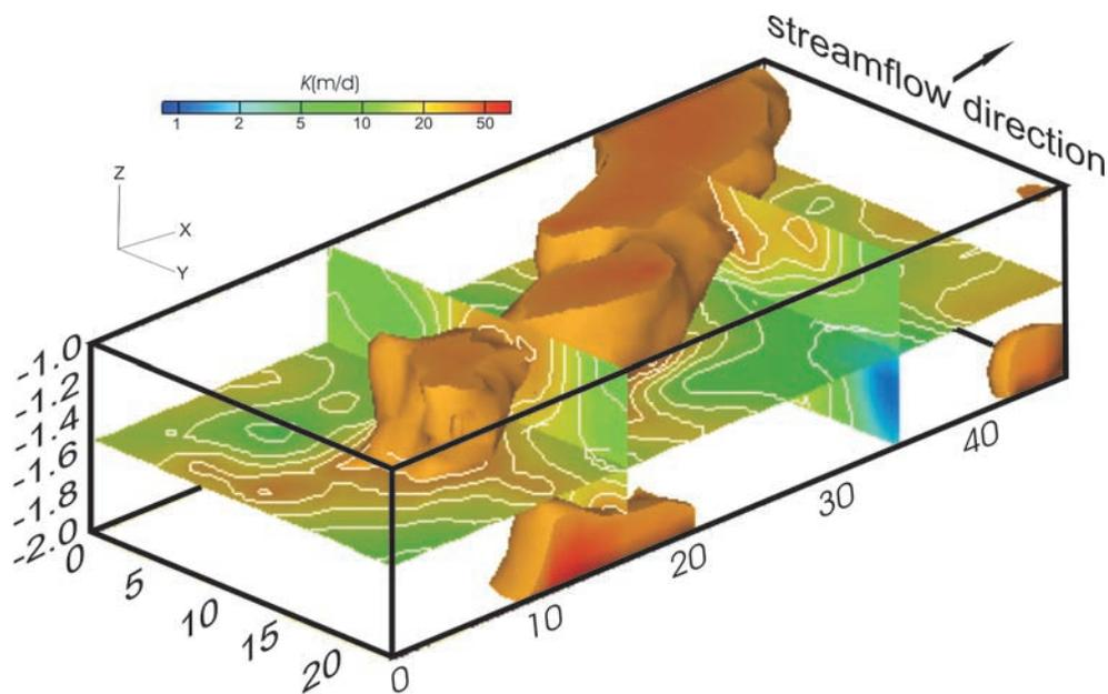
**Figure 7.** Three-dimensional hydraulic conductivity field generated through kriging of  $K$ . Shaded arcuate region corresponds to  $K$  of  $\geq 30$  m/d. Note vertical exaggeration:  $10\times$  and that inset color legend is logarithmic.  $K$  isoline interval on sections is 5 m/d. Axes are in meters.
