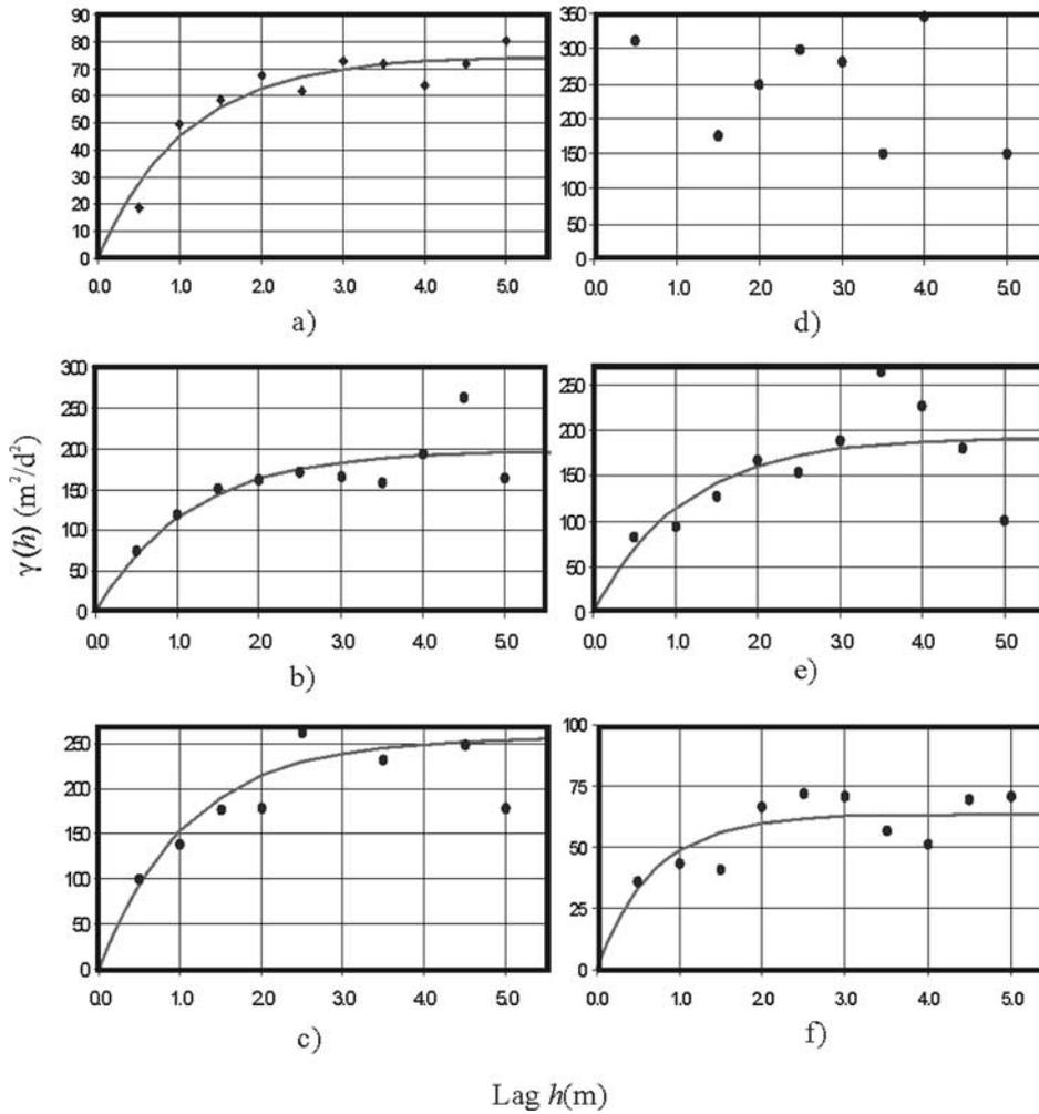
**Figure 9.** Transverse directional variograms and fitted exponential models for different depths: (a) 1.1 m; (b) 1.3 m; (c) 1.5 m; (d) 1.7 m (no variogram model was fit here due to poor definition of spatial structure); (e) 1.9 m; (f) 2.1 m.
