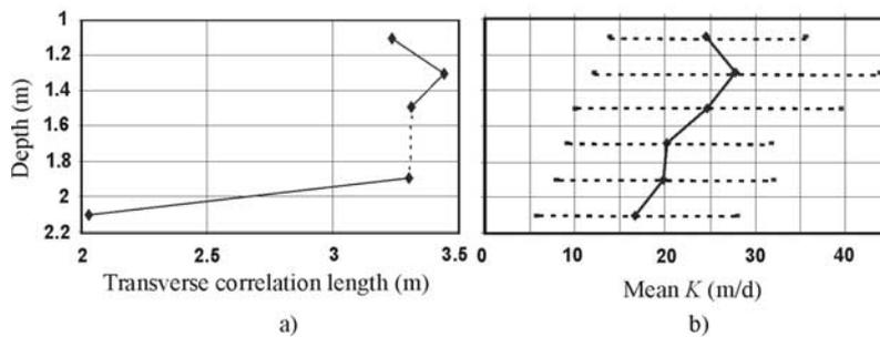
**Figure 10.** Statistical properties of *K* at various depths: (a) transverse correlation length, (b) mean *K* at each depth interval (with one standard deviation). No transverse correlation length was determined for the interval at 1.6 m–1.8 m due to poor definition of spatial structure (see Figure 9d).
