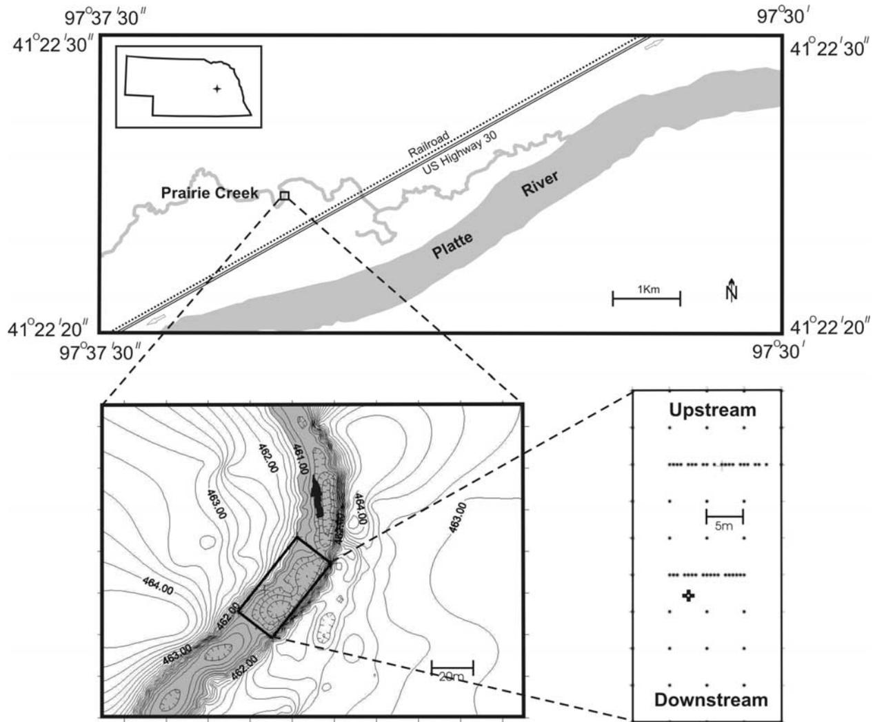
**Figure 1.** Topographic map of the Prairie Creek test site, Nebraska. Solid circles denote location of injection tests in blown-up grid. The open circle indicates location of coupled injection tests and slug tests, and the four surrounding squares are core locations.
