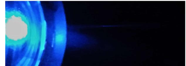
Directly superimposing two laser beams could not produce a viable, noticeable voxel. Angles larger than close to parallel mathematically only increased brightness of the voxel by 7% (See Figure 1).
