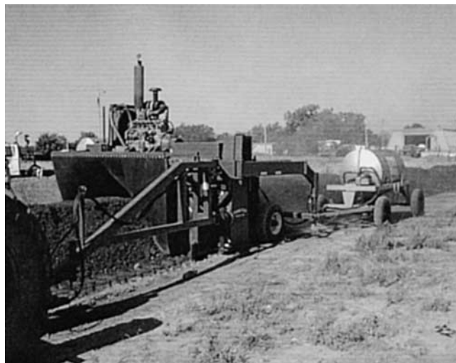
Fig. 1. Soil mixer and water tank being pulled through a soil windrow.
