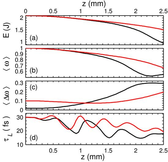
Fig. 2. Evolution of (a) laser pulse energy; (b) mean frequency (in units of  $\omega_0$ ); (c) RMS bandwidth (in units of  $\omega_0$ ); (d) pulse length computed from the  $\zeta$ -variance of the energy density on axis. (WAKE simulations.) Black – the reference case; red – the NCP in a channel. The pulse propagates towards positive  $z$ . The chirp and channel together reduce depletion, frequency red-shift, spectral broadening, and contraction of the pulse (cf. also Fig. 3).
