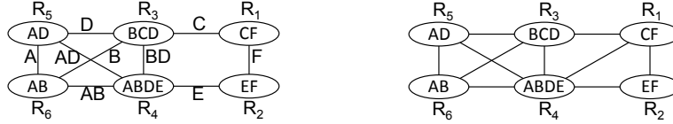
Figure 2: Triangulating a dual graph.
