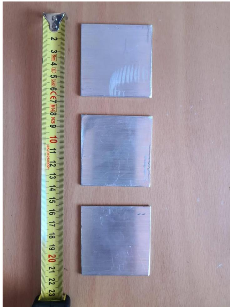
Figure 3-3 The aluminum sheets for preparing the sandwich panel skin
