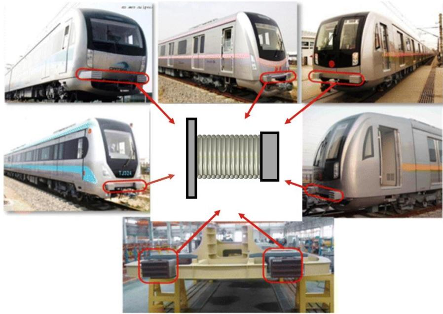
Figure 4-1 Application of Double-sided composite corrugated tube in railway application [54]
