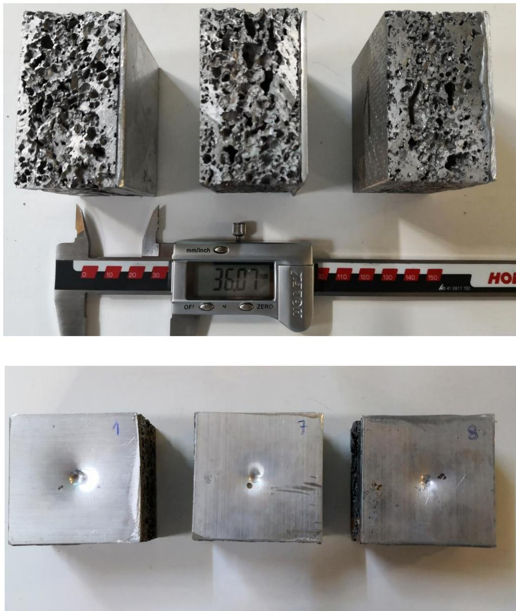
Figure 3-13 The cross section of samples with core thickness of 35 mm (top); the samples after impact tests (bottom)
