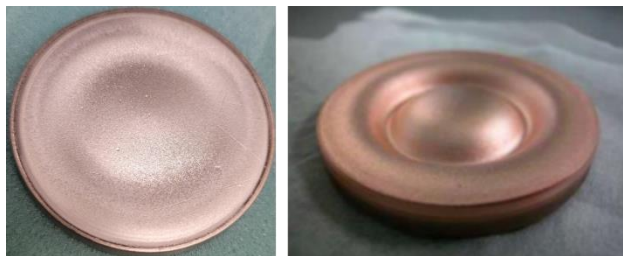
Figure 24 Titanium (left) and copper (right) dc magnetron sputtered targets with the "racetrack"
